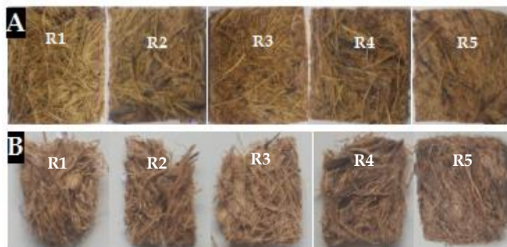
Figure 9. Biodegradation Test Sample (a) Sample before biodegradation test and (b) Sample after biodegradation test
