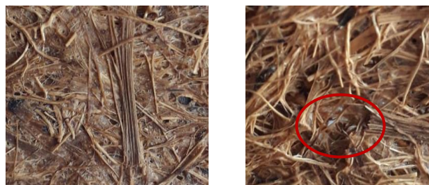
Dispersion Regular Irregular Dispersion Figure 5. Appearance of Fiber Dispersion in Biodegradable Pots
